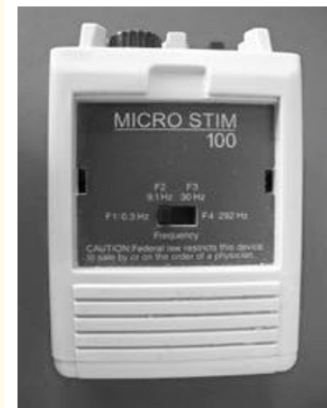
Figure 1: Phase one microcurrent machine using 4 basic Nogier frequencies.
