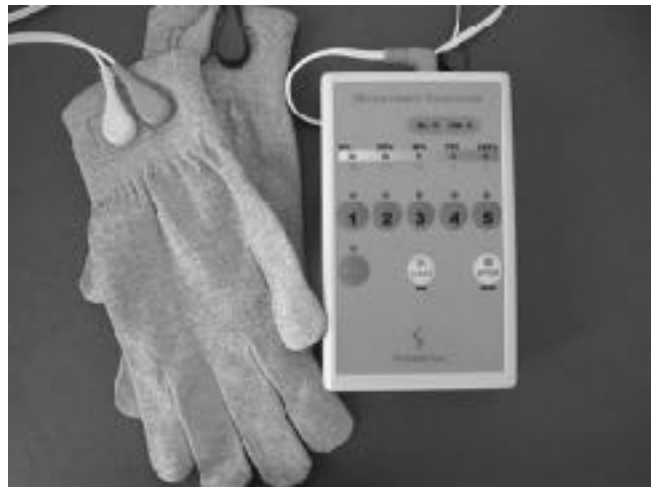
Fig. 3: Phase two microcurrent machine customized able to program frequency
